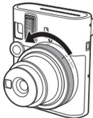
If the camera malfunctions, remove the batteries while the power is on and then reinsert them to reset the camera.
