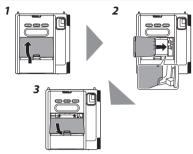
Push up on the battery cover lock and remove the battery cover. Align the battery correctly so that the indentions on the side of the battery match the terminals inside the chamber (as indicated above). Slide the battery in from left to right, and close the lid.
