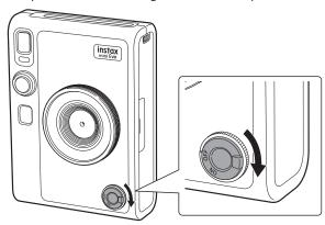
Turn the power switch to the left to turn off the power.
