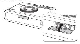
• To remove the memory card, push the card in with your finger and then release your finger gently. The card will be unlocked and is ready to be removed.
