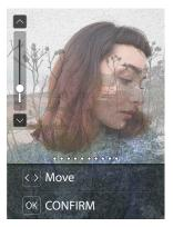
When you press of or on the zoom in/out screen, the screen switches to the move screen, and you can press of to move the screen position. To return to the zoom in/out screen, press (Back).
