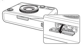
2 Fully insert the memory card into the camera in the correct orientation as shown below until you hear a "click."
