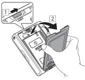
**2** Grasp the rectangular holes on the film pack, then pull film pack out from the camera. Properly dispose of used film pack.
