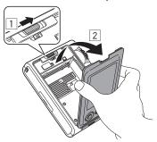
2 Insert an INSTAX MINI instant film pack by aligning the yellow marks.
