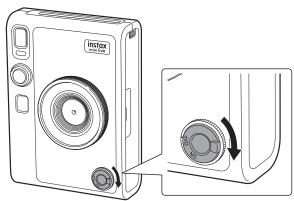
To turn the camera off, turn the power switch anticlockwise.
