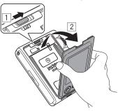
**2** Grasp the rectangular holes on the film pack, then pull film pack out from the camera.
