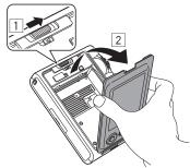
2 Insert film pack by aligning the yellow marks.
