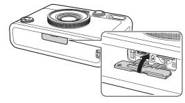
• To remove the memory card, push the card in with your finger and then release your finger gently. The card will be unlocked and ready to be removed.
