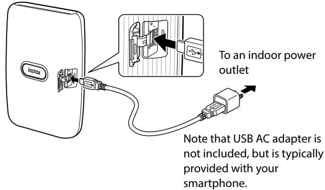
Connect the printer with a USB AC adapter supplied with your smartphone (not included with INSTAX Mini Link printer) using the supplied USB cable, then connect the USB AC adapter to an indoor power outlet.
