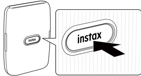
Press and hold the Power button for approximately 1 second to turn the printer on or off.
