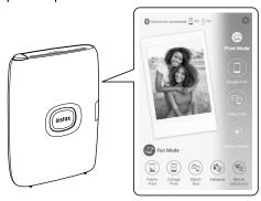
Lay the printer down with the Power button facing up to switch to Fun mode.
