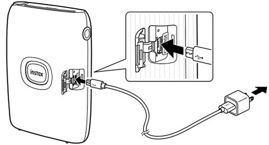
Connect the printer using the supplied Micro USB cable to a USB AC adapter (supplied with your smartphone) then connect the USB AC adapter to an indoor power supply.
