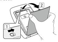
**2** Grasp the rectangular holes on the film pack, then pull film pack out from the printer. Properly dispose of used film pack.
