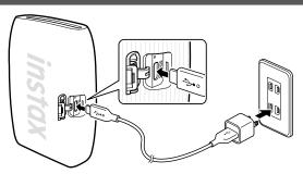
Connect the printer with a USB AC adapter (sold separately) using the supplied USB Type C cable, then connect the USB AC adapter to an indoor power outlet. A USB AC adapter is not included with the INSTAX MINI LINK 3 Smartphone printer (though it may have been supplied with your Smartphone).
