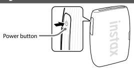
Press and hold the Power button for approximately 1 second to turn the printer on or off.
