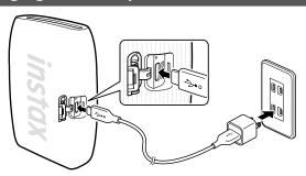
Connect the printer using the supplied USB Type-C cable to a USB AC adapter (supplied with your Smartphone) then connect the USB AC adapter to an indoor power supply.
