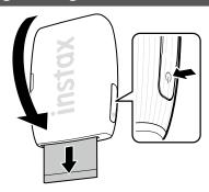
The last image printed can be reprinted by turning the printer over with the film ejection slot facing downwards and pressing the power button.
