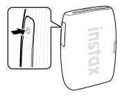
Press and hold the Power button for approximately 1 second to turn the printer on or off.
