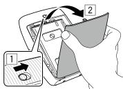
**2** Grip the rectangular holes on the film cartridge and remove the empty film cartridge.
