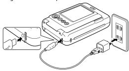
Connect the camera and a USB AC adapter supplied with your Smartphone using the supplied USB Type C cable, then connect the USB AC adapter to an indoor power outlet.
