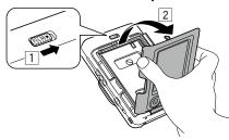
**2** Grasp the rectangular holes on the film pack, then pull the film pack out from the camera.
