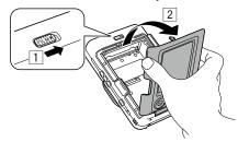
2 Insert a film pack by aligning the yellow marks.
