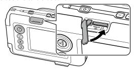
• When removing a memory card, push against the memory card with your finger and slowly release your finger from the card. The lock is released and the memory card can be removed.
