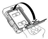
4 Remove the black protective film cover that is ejected, automatically.
