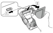
**2** Insert a film cartridge by aligning the yellow marks.
