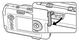
2 Insert the memory card all the way until a click is heard. Ensure the correct orientation is used as shown below.
