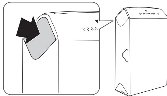
2 Select **instax PRINTER PRINT** in the camera playback menu. The camera will connect to the printer.
