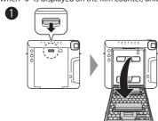
Press the back cover lock down to open the back cover.
