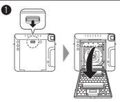
Press the back cover lock down to open the back cover.
