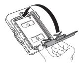
4 Remove the black film cover that is automatically rejected
