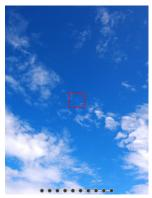
The red AF Frame displays on the LCD monitor. Either change the composition or use the AF/AE Lock. (See p. 16)
