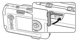
• When removing a memory card, push the memory card with your finger and slowly release your finger. The lock is released and the memory card can be removed.
