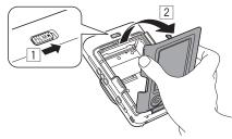
2 Insert the INSTAX Mini Instant Film Pack by aligning the yellow marks
