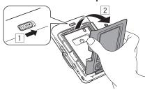
**2** Grasp the rectangular holes on the INSTAX Mini Instant Film Pack, then pull the film pack out from the camera
